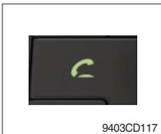
① When established bluetooth connection is made between this audio unit and the cellular phone, bluetooth icon on the display appears and then the display shows HF/AV CONN when handsfree & AV profile is connected.
