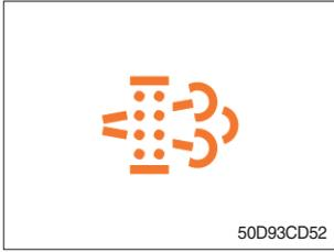
① This warning lamp lights ON when the SCR cleaning is needed and lamp flashes when manual SCR cleaning is activated as table below.
